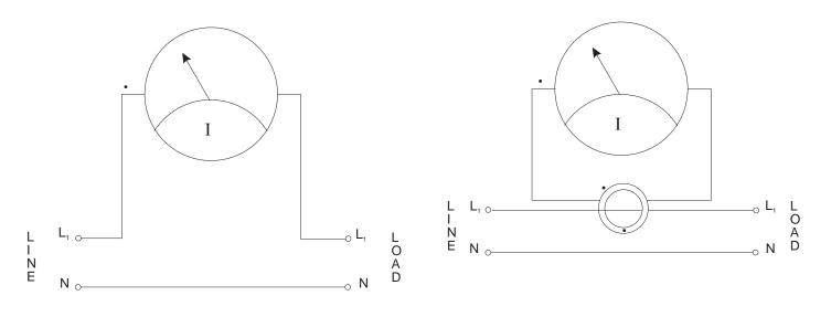
a) Current Meter, Typical Installation, no Current Transformer b) Current Meter, Typical Installation, with Current Transformer
