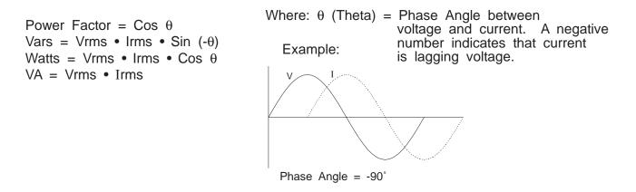
Figure 12 Phase, Power Factor, and VAR Conventions Employed by the 1040C Panel Meter Calibrator
