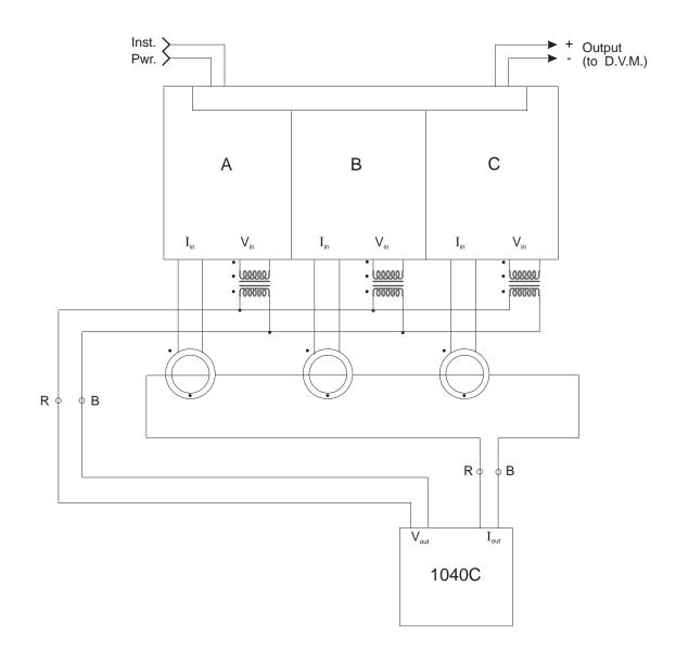
Figure 10 Calibration Connections for 3-Element Watt Transducer. Current and Potential Transformers are included for reference.
