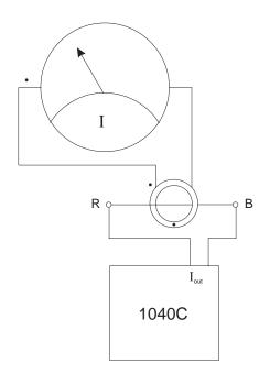
b) Current Meter Calibration Connections, with Current Transformer
