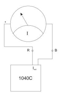
a) Current Meter Calibration Connections, no Current Transformer
