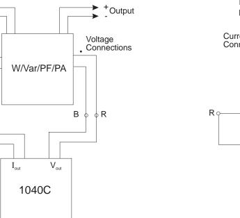
c) W/Var/PF/PA Transducer Calibration Connections, no Current or Potential Transformers
