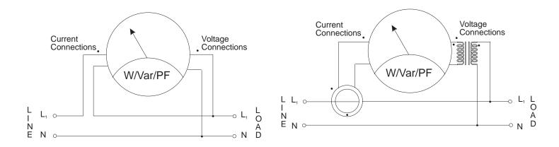
a) W/Var/PF Meter, Typical Installation, no Current or Potential Transformers b) W/Var/PF Meter, Typical Installation, with Current and Potential Transformers
