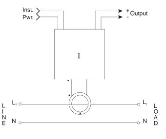
d) Current Transducer, Typical Installation, with Current Transformer
