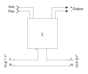
c) Current Transducer, Typical Installation, no Current Transformer
