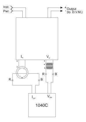
b) Typical Calibration Connections
