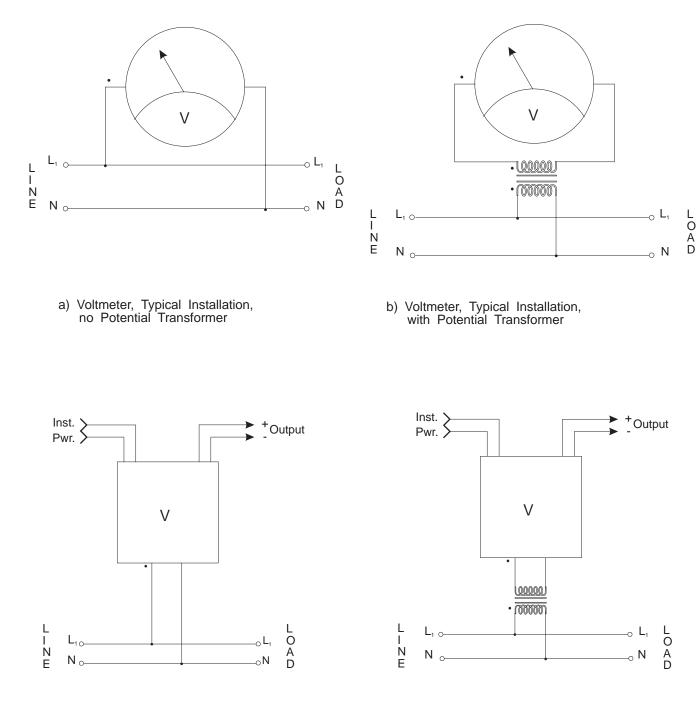
c) Voltage Transducer, Typical Installation, no Potential Transformer d) Voltage Transducer, Typical Installation, with Potential Transformer
