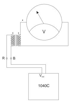
a) Voltmeter Calibration Connections, no Potential Transformer
