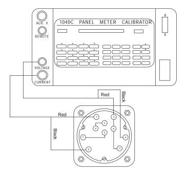
4 WIRE, 3 PHASE, 2 1/2 ELEMENT VARMETER YOKOGAWA 10329 \_\_\_\_\_
