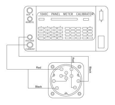
4 WIRE, 3 PHASE POWER FACTOR METER YOKOGAWA 103472 \_\_\_\_\_
