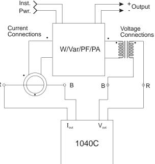
d) W/Var/PF/PA Transducer Calibration Connections, with Current and Potential Transformers
