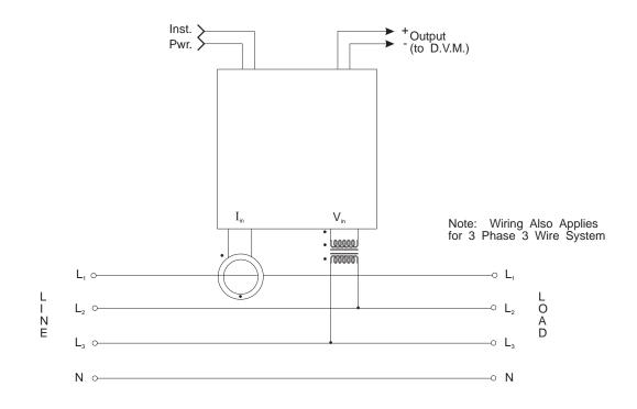
a) Typical Circuit Connections
