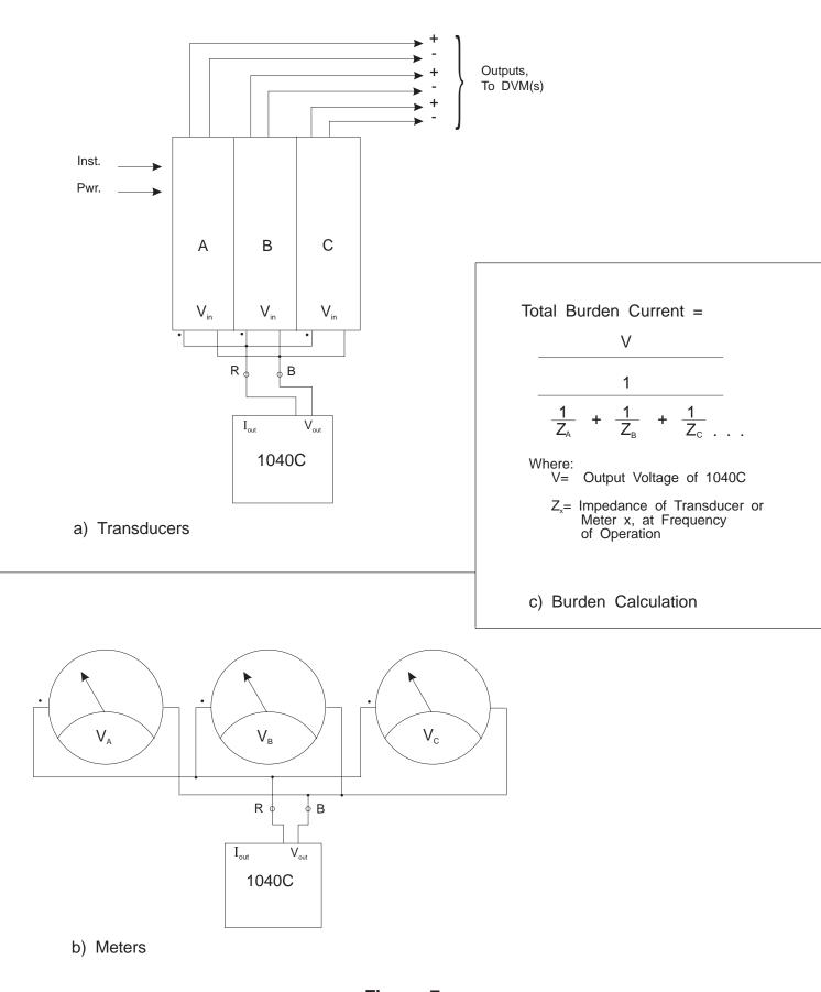
Figure 7 Calibration of Multiple Voltage Transducers or Meters
