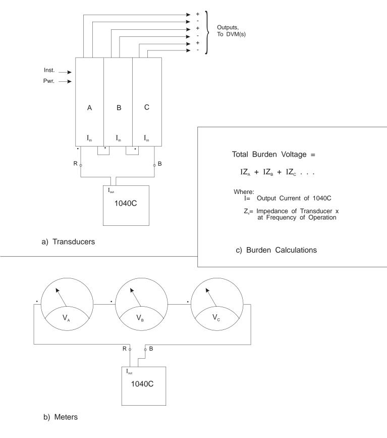
Figure 8 Calibration of Multiple Current Transducers or Meters
