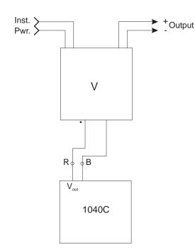
c) Voltage Transducer Calibration Connections, no Potential Transformer
