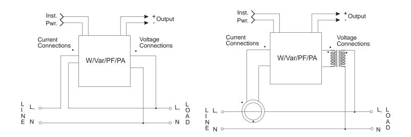
c) W/Var/PF Transducer, Typical Installation, no Current or Potential Transformers
