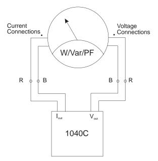
a) W/Var/PF Meter Calibration Connections,
